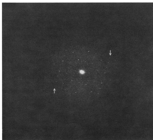
FIGURE 3 Optical diffraction pattern of an image of a frozen hydrated gp32*I crystal. The crystal was frozen in liquid ethane and imaged at 130°K. The highest resolution reflection (arrow) is (3, 4) at 11.1 Å.
